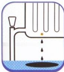
'Pin holed' radiators
